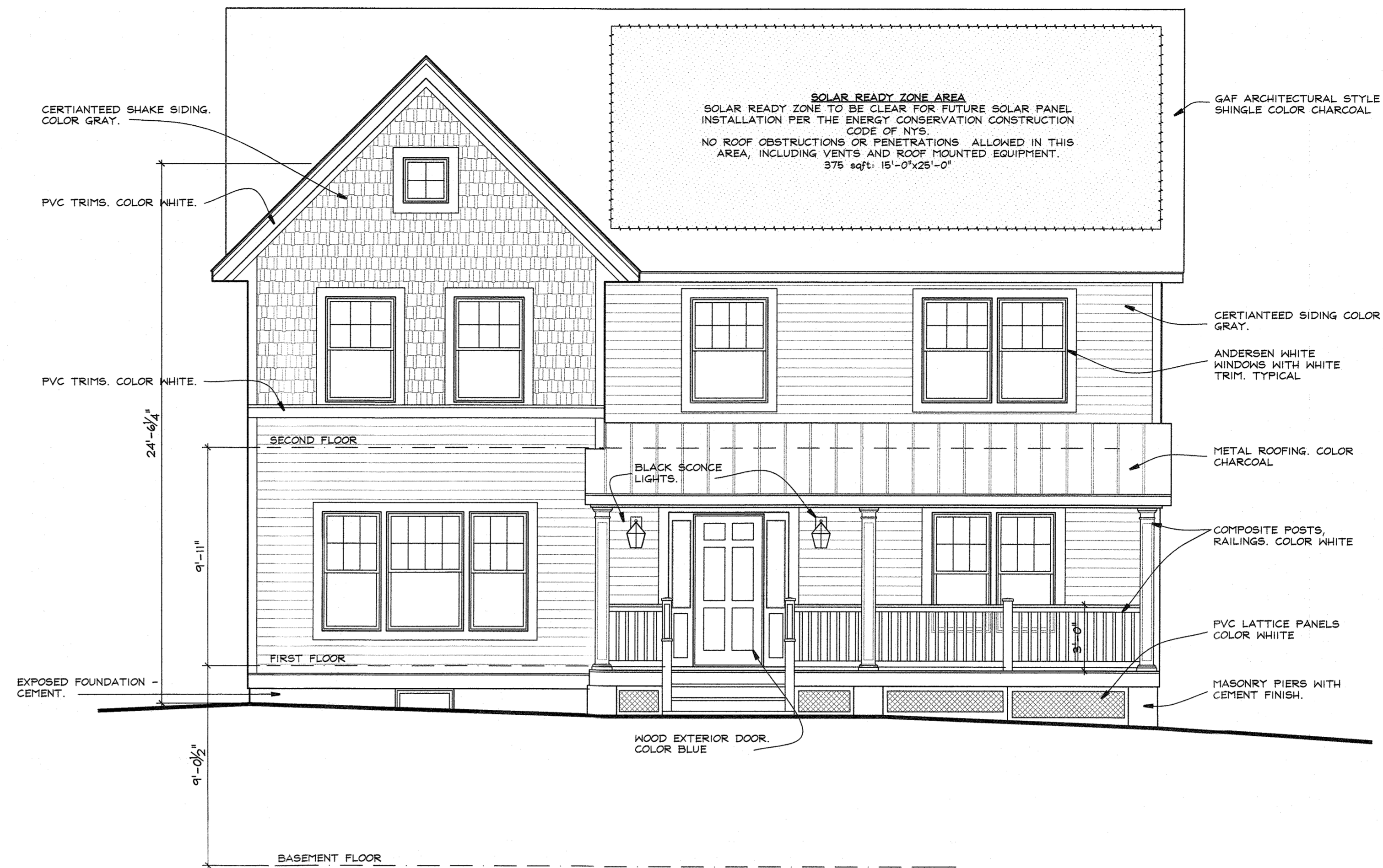
A FRONT (SOUTH) ELEVATION A3 1/4" = 1 FOOT
