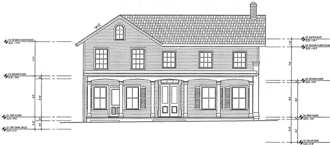
1 EXISTING FRONT(NORTH) ELEVATION SCALE: 1/4"=1'-0"
