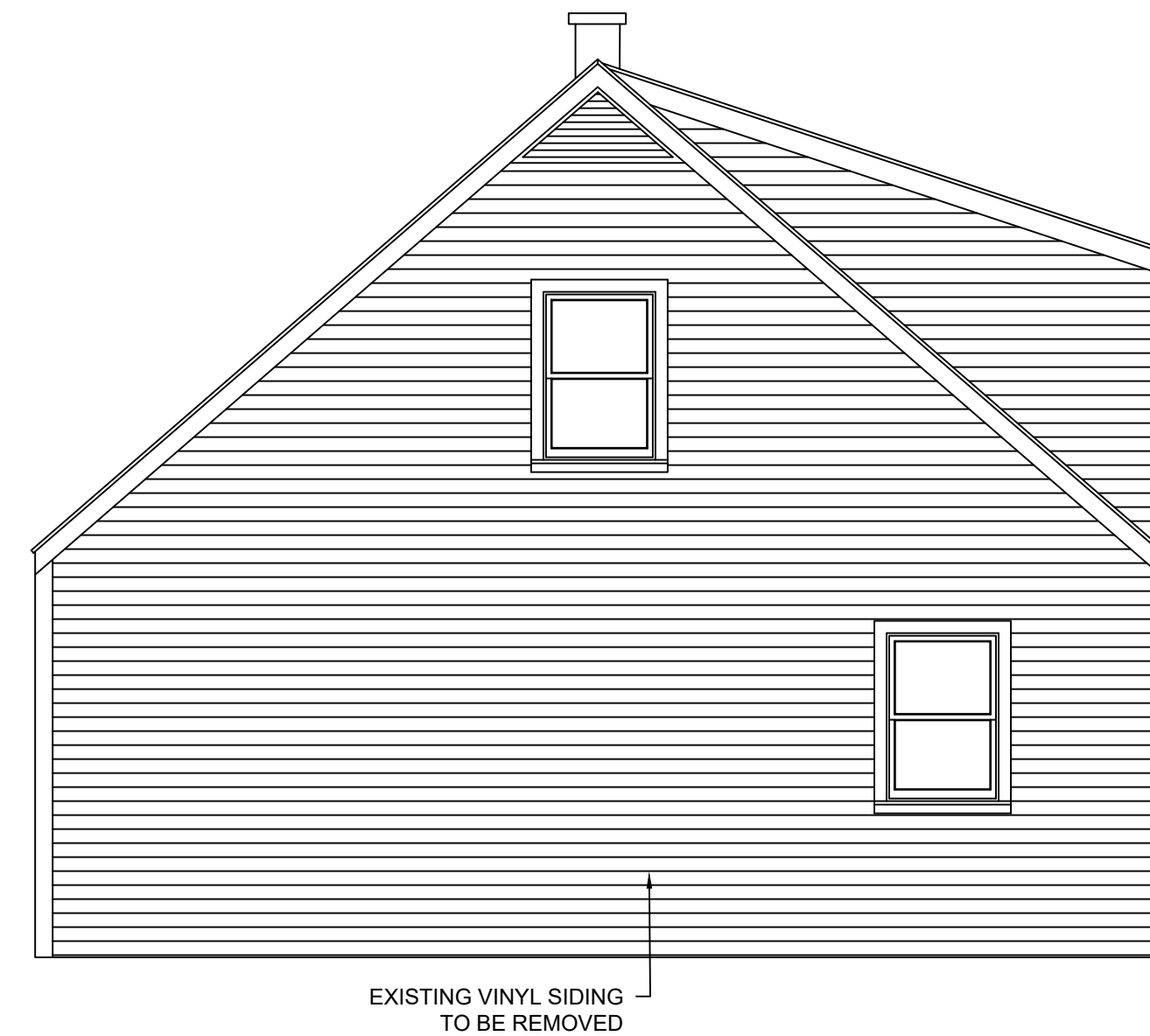
2 A-3 EXISTING SIDE ELEVATION (EAST) SCALE: 1/4" = 1'-0"
