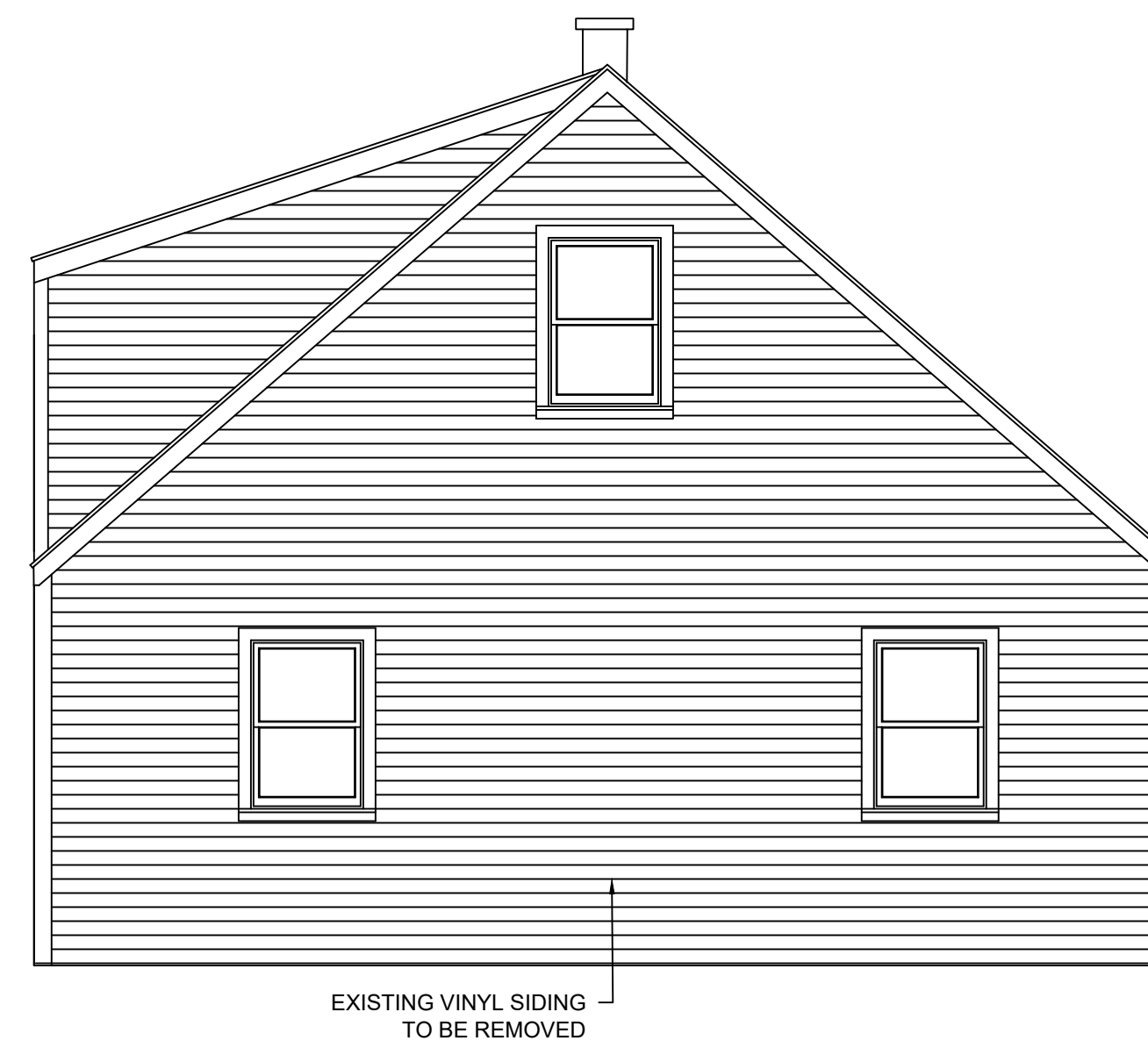
4 A-3 EXISTING SIDE ELEVATION (WEST) SCALE: 1/4" = 1'-0"
