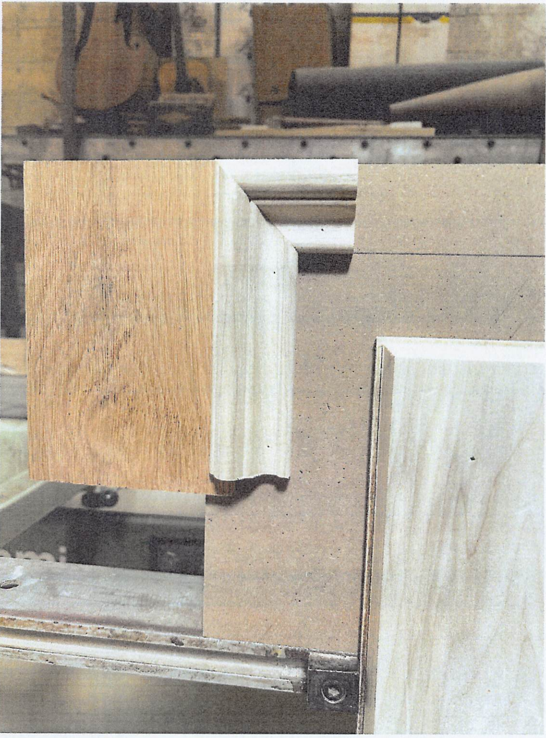
DETAIL - Frost Door Raised Panel
