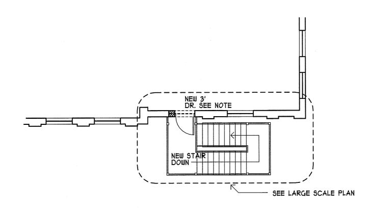
PARTIAL SECOND FLOOR PLAN (WORK AREA #1) SCALE: 1/8" = 1'-0"
