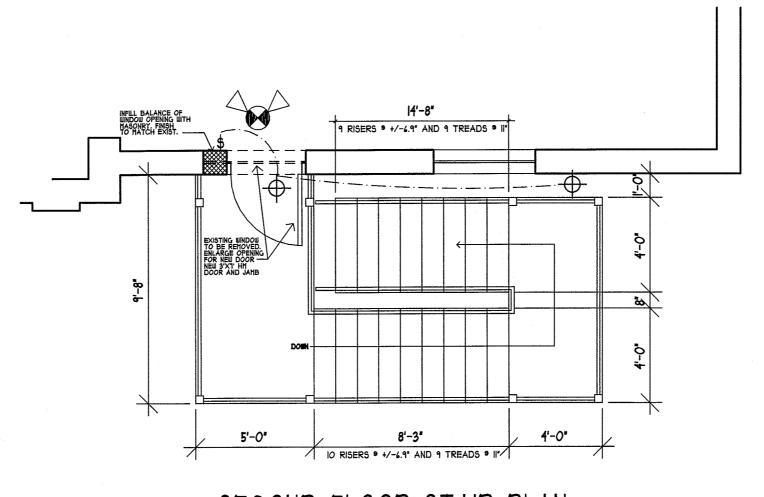
SECOND FLOOR STAIR PLAN (WORK AREA #1) SCALE: 1/4" = 1'-0"
