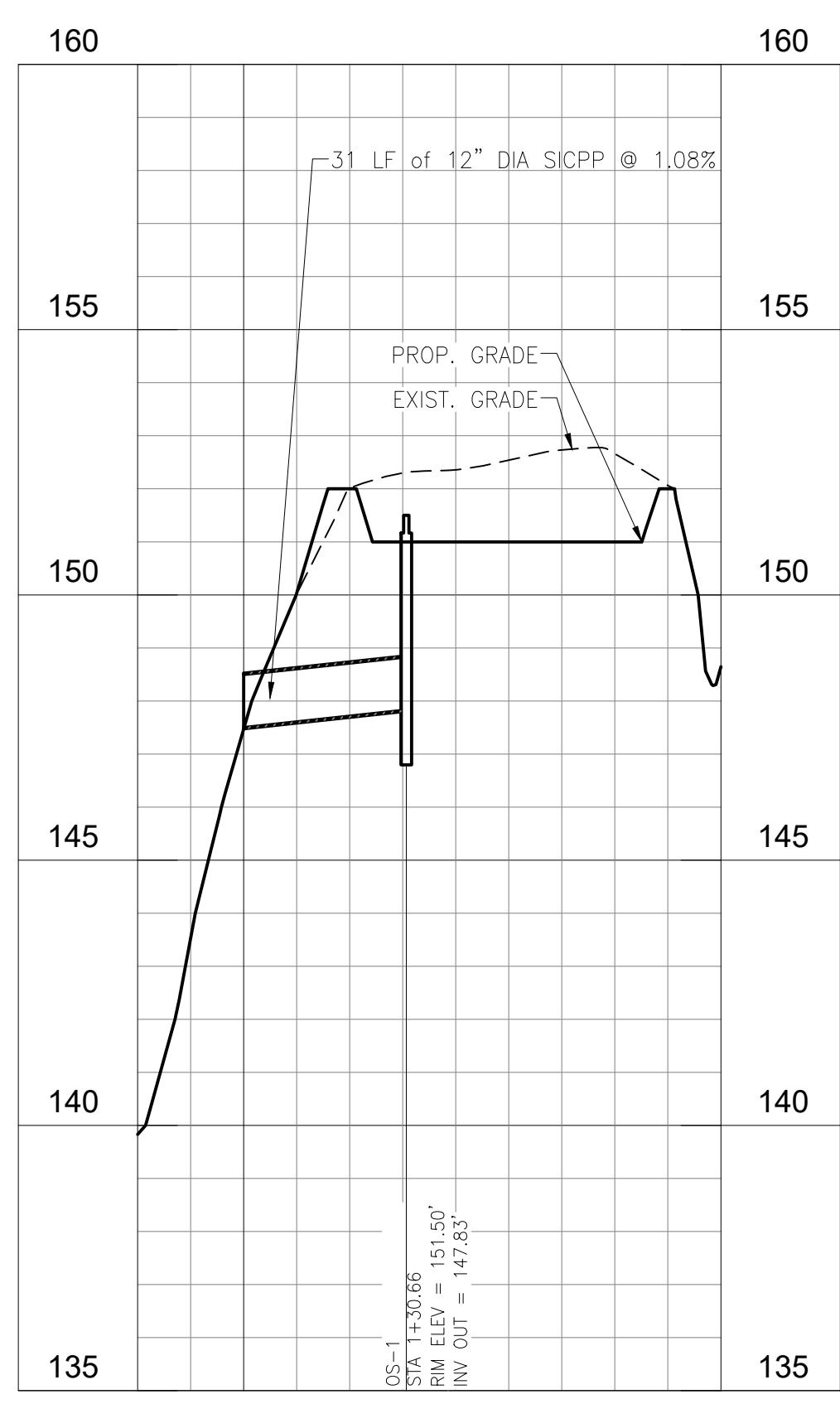
BIO-RETENTION AREA #1 PROPOSED STORM DRAIN HORIZONTAL: 1" = 30' VERTICAL: 1" = 3'
